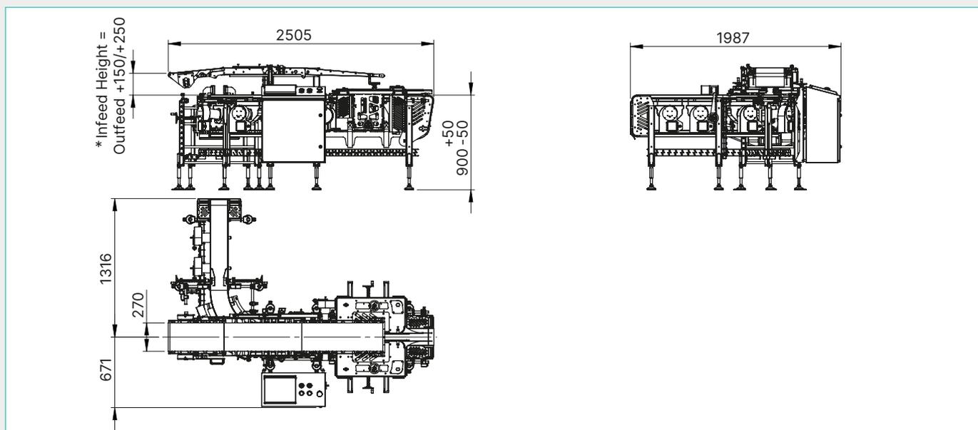
Specifications and photos are intended as a guide and can be changed by QUPAQ without notice. We make reservations for misprints and typing errors. The illustration and specifications are of the QUPAQ Flex Loader 150F. Item no. 90000252.
